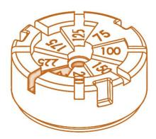
Typically, the relief valve leaves the factory set at 150 PSI. You must look at the settings prior to use to make sure that it is set correctly for your application and if adjustment is needed do so prior to putting into service.
