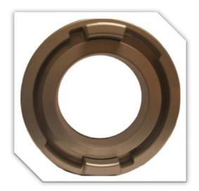
**Description:** Open Bore Storz is a quick connecting device that allows you to quickly connect up to a fire hydrant without threading on an adapter at the scene. This design allows you to connect up seamlessly to a hydrant. This item would need a blind cap with it when purchasing to seal the open hole in the middle.
