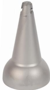
The **Critical Valve Lock (V-Lock)** is a patented water distribution security device that is designed to limit the access of operating nuts on underground gate valves in the water distribution system. The V-Lock is lowered onto a critical gate valve to provide either a long or short term lock out / tag out system of the operating nut. The V-Lock is designed to secure the on or off position of gate valves in critical water zones where control is required.
